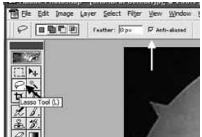
Figure 5. Steps to turn off anti-aliasing. Click on the lasso tool (black arrow) then uncheck the anti-aliasing box, which will appear at the top of the working window (white arrow).
