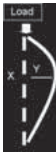
Figure 4. The bending moment and lateral displacement. The bending moment at any point (X) is the product of lateral displacement (Y) and the load. As the lateral displacement increases, the propensity for further buckling increases.
